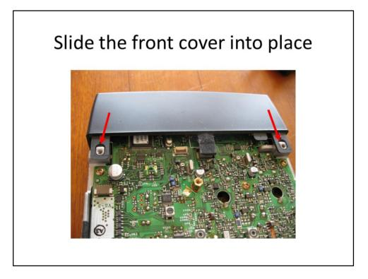
This will cover the battery and snaps into place on the four corners. Be sure to check the alignment of the front connectors.
