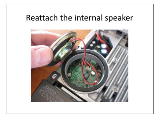
Position the rubber cushion ring <u>before</u> plugging in the speaker leads. Then the two covers go back on with the remaining 11 screws and you're done.
