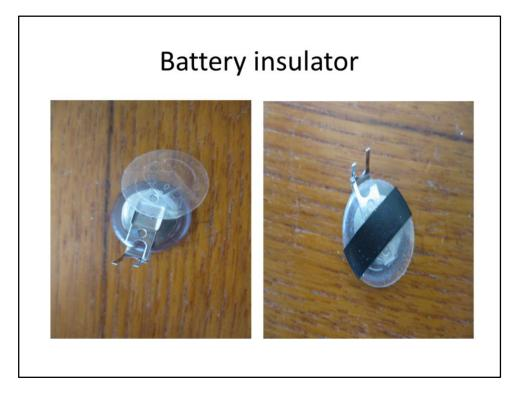
Now the battery rests on an integrated circuit so as a precaution there's a plastic spacer between them. The adhesive is pretty weak after 15 years so I've cut a piece of electrical tape to hold it in place. Now's a reeeally good time to break out your DVM and double-check that the battery voltage is at least 3 volts DC!
