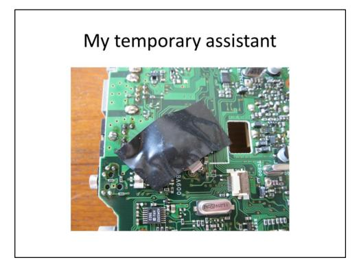
The electrical tape is ugly but temporary. You want to hold the battery in a position so that the leads just barely stick through the other side. Commercial PCBs almost always have plate-through holes so it won't take much solder to tack these leads down.
