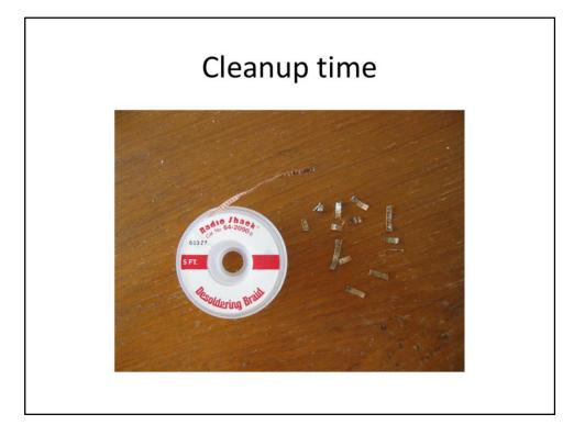
Each time you use copper desoldering braid cut off the end piece that soaked up the solder. Don't try to be cheap here. You don't want any excess solder wicking onto the board.
