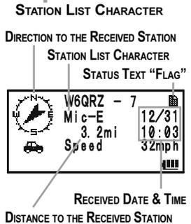
When the “Status Text” is included in the Mic Encoder Station Beacon, the **🚗** icon appears at the upper right corner of the display.
