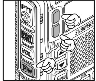
Press and hold in the **A** or **B** key for 1/2 seconds to switch to Mono Band Operation. During Mono band operation, you may change the display between “*double-size character*” and “*large character*” by pressing the **A/B** key.
