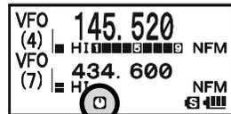
Just press and hold in the **(PWR)** switch for 2 seconds to turn the transceiver back on after an APO shutdown, as usual.
