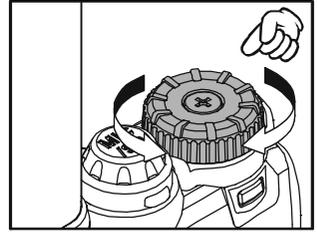
If you press the **[BW]** key briefly, then rotate the **DIAL** knob, frequency steps of 1 MHz will be selected. This feature is extremely useful for making rapid frequency excursions over the wide tuning range of the **VX-8DR/DE**.
