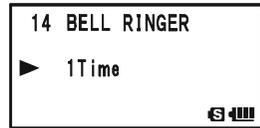
When you are called by a station whose transceiver is sending a CTCSS tone, DCS code, or CTCSS tone pair which matches that set into your Decoder, the Bell will ring in accordance with this programming.
