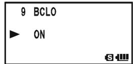
To disable the BCLO feature, just repeat the above procedure, rotating the **DIAL** knob to select "OFF" in step 4 above.
