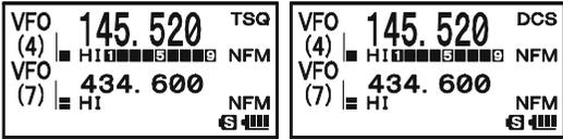
2. Press the **[F/W]** key, then press the **CODE 2 ABC** key to recall the Set Mode Item 99: TONE FREQUENCY when CTCSS is selected, or Menu Item 26: DCS CODE during DCS operation.
