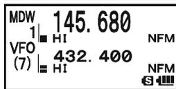
The receiving time interval (ratio) between the current channel (or VFO frequency) and Priority channel may be customized via Set Mode Item 72: PRI TIME.
