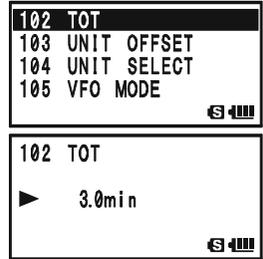
To disable the Time-Out Timer, just repeat the above procedure, rotating the **DIAL** knob to select "OFF" in step 4 above.
